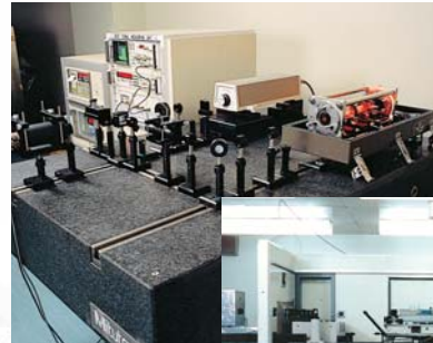
Iodine Absorption Stabilized HE-Ne Laser as the standard for length measurement (at Tsukuba Calibration Center)
