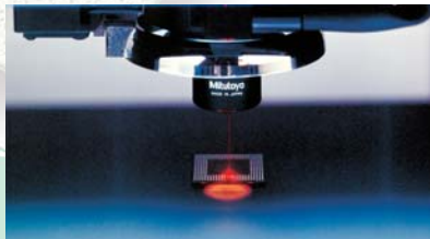
Height measurement of the terminals on the connector
