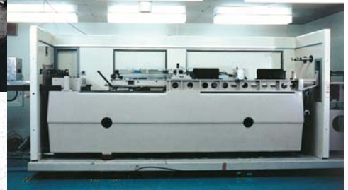
Interferometer as the standard for Linear Scale calibration (at the Kiyohara plant)
